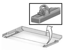
The loop of the D-ring slider must be facing inward towards the storage area and the ring must be in the up position for proper usage.
